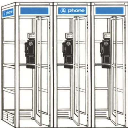
Correct markings for 3 booths
