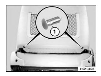
Release clips (1) with side cutting pliers.
