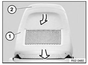
Lever out rear panel (1) at bottom towards rear and pull out towards bottom from backrest frame (2).
